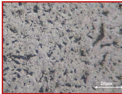
Fig. 19 Unetched Optical Micrograph of Al-Al 2 O 3 Composite (A4) at 500X (Hold time 3 h) at 850 0 C.
