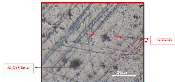
Fig. 8 Unetched Optical Micrograph of Al-Al 2 O 3 Composite at 500X, Holding 3h, 4 times Stirred Each after 45 Min Interval at 850 °c.
