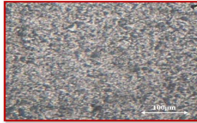
Fig. 18 Etched Optical Micrograph of Al-Al 2 O 3 Composite (A4) at 100X (Hold time 3 h) at 850 0 C.
